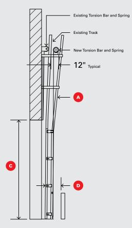
NOTES: A torsion bar support is required on all doors 10' or wider. Dual track cannot be used if existing door has outside pull cables. The Rasco door has outside pull brackets/cables.
